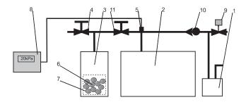
FIGURE 1. Schematic diagram of the experimental stand: 1 - vacuum pump, 2 - main tank, 3 - basic tank, 4 - ball valve, 5 - sensor of the pressure, 6 - sample treated by vacuum pressure, 7 - mesh preventing the sample ingestion, 8 - vacuum pressure gauge, 9 - electro valve, 10 - check valve, 11 - valve.
