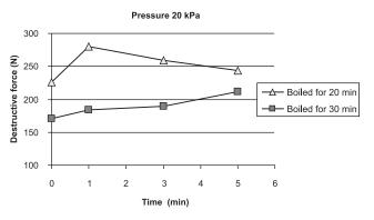
FIGURE. 4. Changes of destructive force for maize seed samples subjected to 20 and 30 min hydro-thermal treatment and vacuum pressure of 20 kPa.
