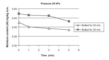
FIGURE. 3. Changes in the moisture content (dry basis) of raw materials subjected to 20 and 30 min hydro-thermal treatment and next to the vacuum pressure of 20 kPa.
