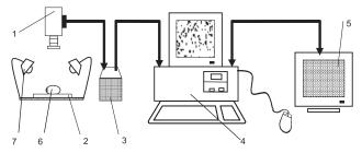
FIGURE 2. Scheme of the SVIST system for computer image analysis: 1 – digital camera, 2 – subject table, 3 – converter, 4 – personal computer, 5 – screen, 6 – sample, 7 – source of light.
