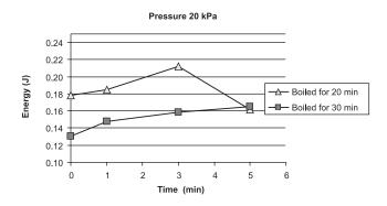
FIGURE. 5. Changes of destructive energy for maize seeds after 20 and 30 min hydro-thermal processing, subjected to vacuum pressure 20 kPa.
